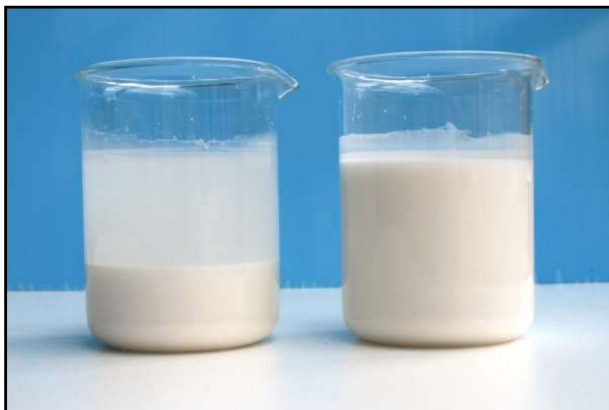
Fresh slurry of limewash ("Kalkmilch"; right) and after about 20 min. time (left): at the bottom the limewash has settled (calcium hydroxide - water—mixture), over it there is the turbid lime water ("Kalkwasser") that you can drop into the aquarium water.
